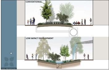
Figure 2. This graphic from the winner of the urban redevelopment design category shows how a conventional vegetated area (top) compares with a low impact option (bottom).
