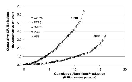
Figure 2. Comparison of Annual Emissions of CF<sub>4</sub> from Primary Aluminium Production Facilities for 1990 and 2000. (IAI, 2001)
