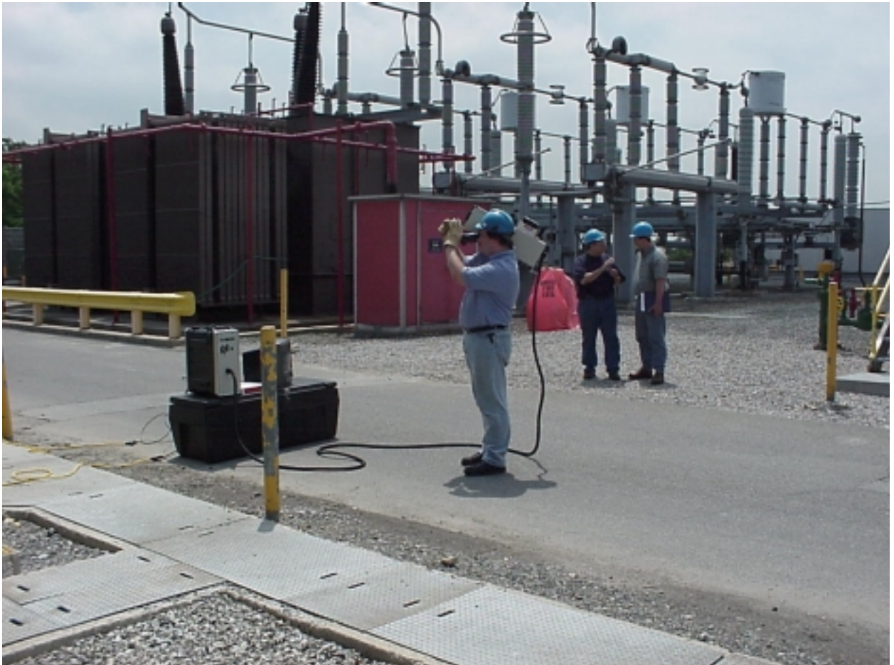
Figure 2. The first of the new-generation laser cameras is undergoing a field trial at Consolidated Edison Co. The operator holds the shoulder unit while the remainder is atop the shipping case.
