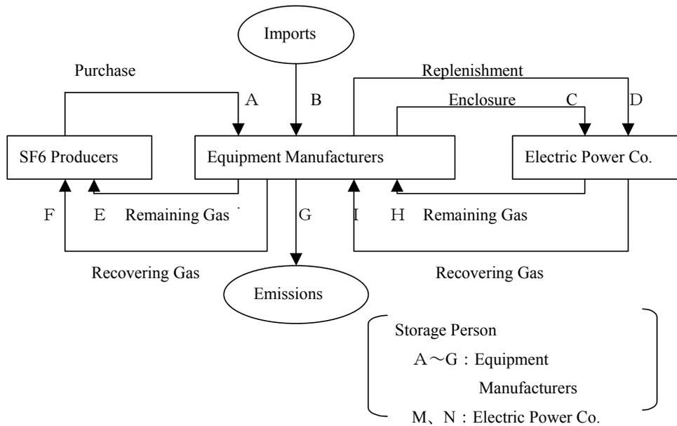
Fig. 3 SF6 flow and control centered on equipment manufacturers
