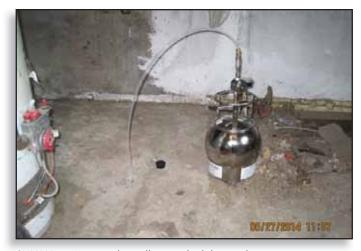
SUMMA canister used to collect a sub-slab sample.
