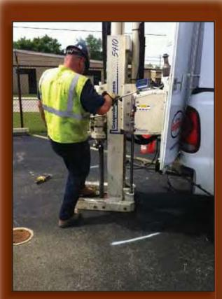
A worker uses direct push technology, or DPT equipment to take samples. DPTs are a category of equipment that push or drive steel rods into the ground. They allow costeffective, rapid sampling and data collection from unconsolidated soil and sediment. A tremendous variety of equipment is available, particularly in the type of attachments used at the end of rods to collect samples and data. These attachments may collect soil, soil gas or groundwater samples.
