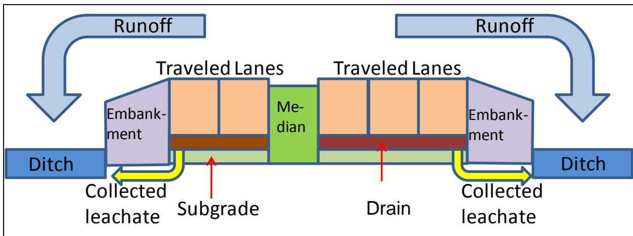
**Figure 4-5. Sample road design cross-section.**
