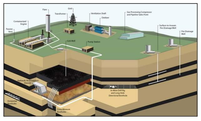
Figure 1. Removal of CMM from Longwall Mines
