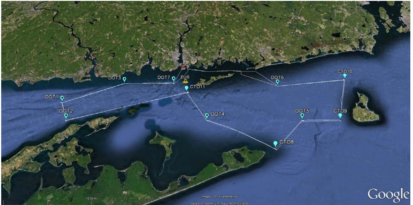
Figure 1. Locations of moored instrument arrays (DOT1-DOT7) and CTD profiles (CTD8-CTD11). LEDG is UConn's New London Ledge Light meteorological station and ELIS is UConn's metocean observation buoy. White line delineates the survey tracks for both days.
