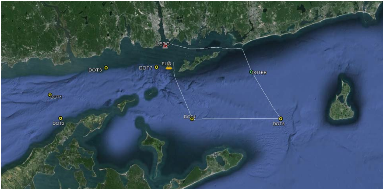
Figure 1. ADCP survey track from December 12 th .. LEDG is UConn's New London Ledge Light meteorological station and ELIS is UConn's metocean observation buoy.
