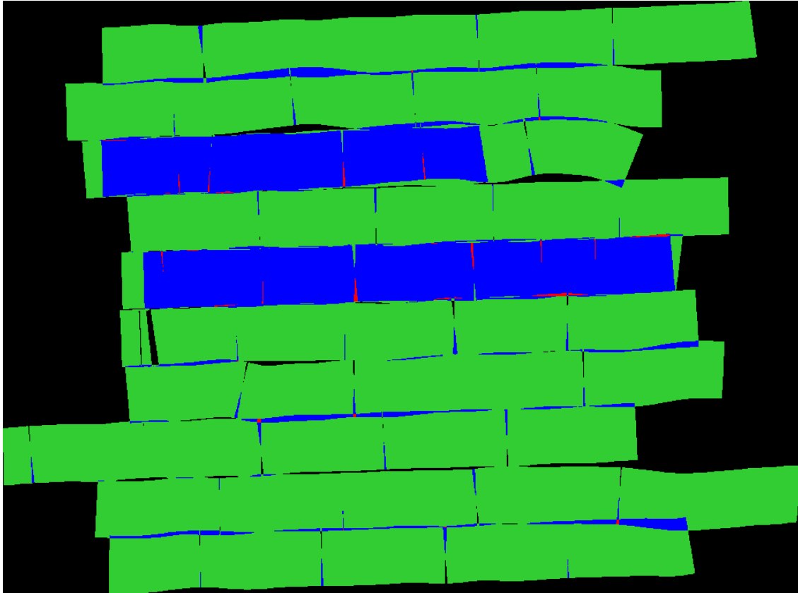
Figure 3.29.1. NLDN_ACT survey data coverage. The green and blue colors indicate survey area with 100% coverage (0% overlap) and 200% coverage (100% overlap), respectively.
