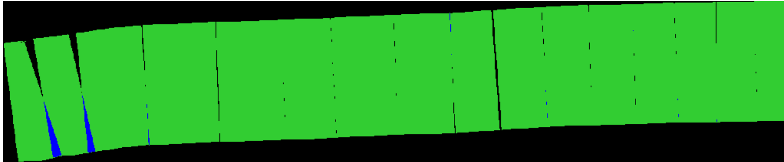
Figure 3.20.1. FISE_SW_ADD2 survey data coverage. The green and blue colors indicate survey area with 100% coverage (0% overlap) and 200% coverage (100% overlap), respectively.
