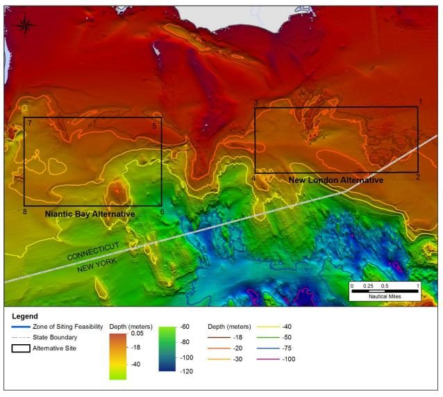
**Figure 3.** Location of the New London and Niantic Bay Alternatives. Coordinates of corner points are presented in Table 1. (Bathymetric data source: Poppe et al., 2011)
