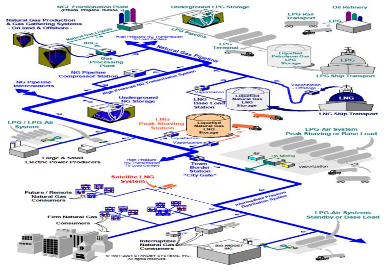
3 From wellhead to burner tip, this graphic shows the pieces and parts of a natural gas energy grid. The sections in orange show a typical LNG peak shaving plant location.
