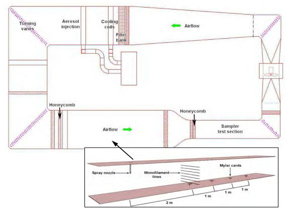
Figure 2. EPA's aerosol wind tunnel (AWT).
