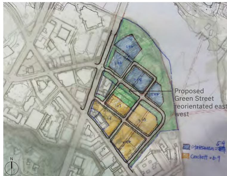
Figure 17 The plan to the left illustrates the revisions proposed to the 2014 street grid. The proposal reorients the “Green Street” feature from its north-south orientation in the 2014 plan to an east-west orientation. The goal of this change is to link the SCW neighborhood from east to west across South Congress Avenue and to reinforce South Congress Avenue as the primary north-south street in the SCW neighborhood and the city.
