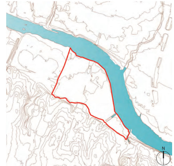
Figure 6 The above diagram illustrates ten foot contour lines over the site, demonstrating its relative flatness.
