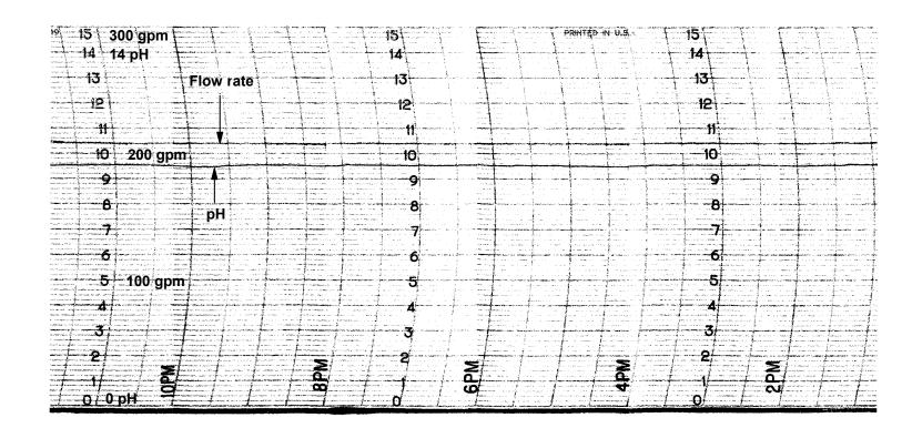
Figure 1. Typical scrubber flow rate and pH.
