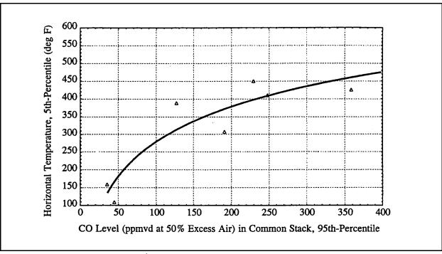
Figure A.16-2. CO Level (95<sup>th</sup> Percentile) in the Common Stack vs. Horizontal Temperature Measurement (5<sup>th</sup> Percentile).
