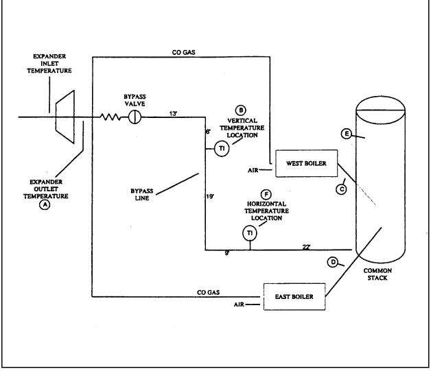
Figure A.16-1. Process schematic.
