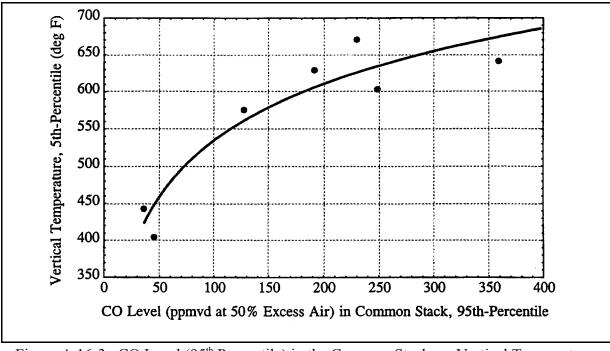
Figure A.16-3. CO Level (95<sup>th</sup> Percentile) in the Common Stack vs. Vertical Temperature Measurement (5<sup>th</sup> Percentile).
