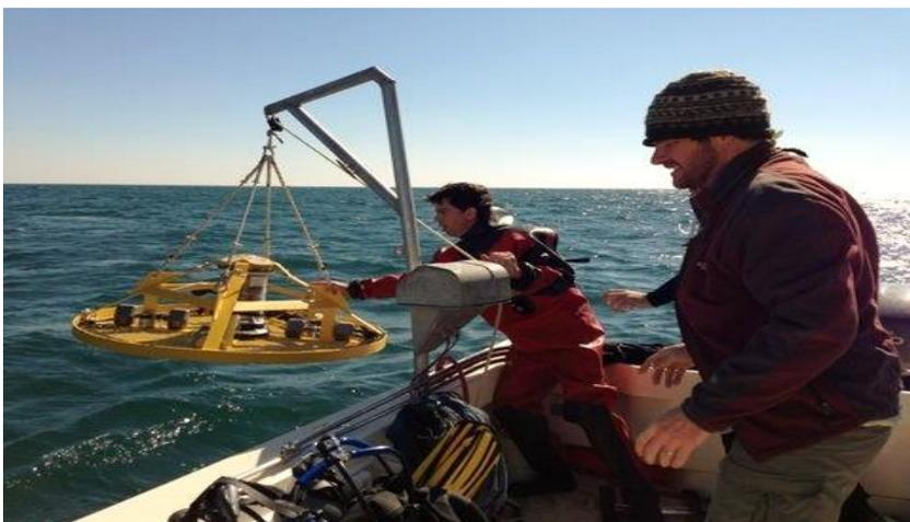
Retrieval of current meters at Ocean Dredged Material Disposal Sites (ODMDS). Acoustic Doppler Current Profiler (ADCP) meter retrieval offshore, Charleston, South Carolina.
