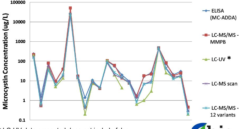
\* LC-UV data presented does not include falsepositives that were eliminated from total (Based on lack of confirmation with LC-MS methods). Sample # 14 was non-detect using LC-UV. Ohio Environmental Protection Agency
