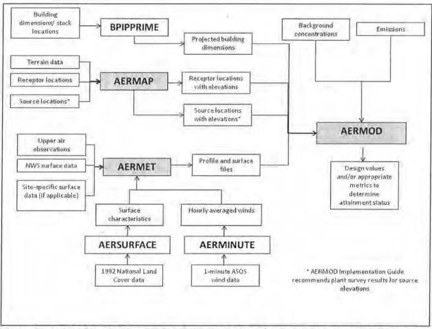
Figure 1. AERMOD modeling system framework. Regulatory components of the system are in gray boxes.
