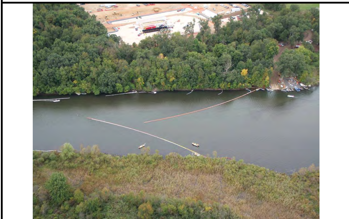
Photo Plate 2: Gate Booming System (also referred to "Open Chevron")
