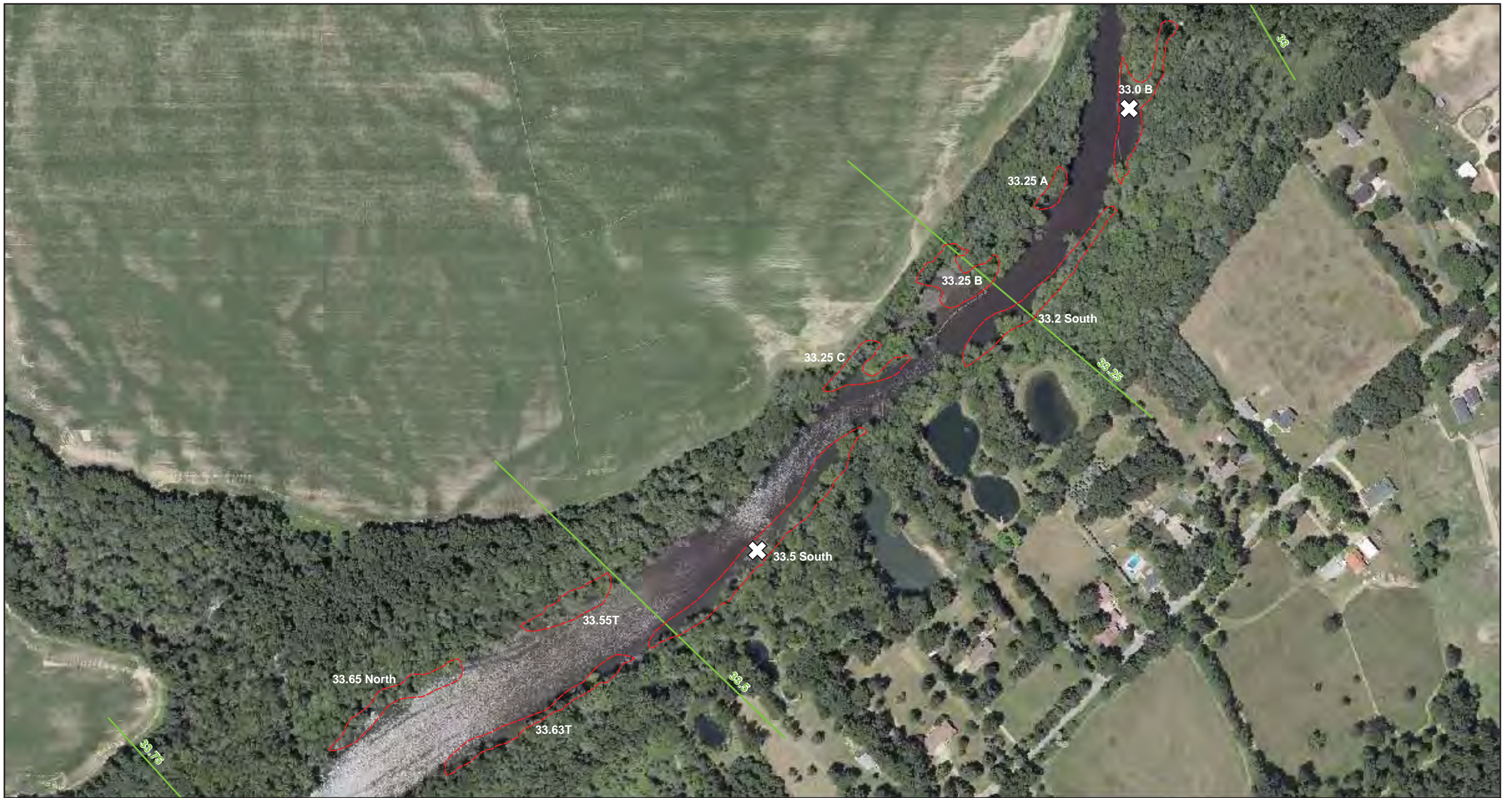
FIGURE 3 PROPOSED CORING LOCATIONS MP 33.10 - MP 33.70 ENBRIDGE LINE 6B MP 608 MARSHALL, MI PIPELINE RELEASE ENBRIDGE ENERGY, LIMITED PARTNERSHIP
