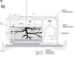
Cross-section detail of tree filter showing engineered soil which filters stormwater
