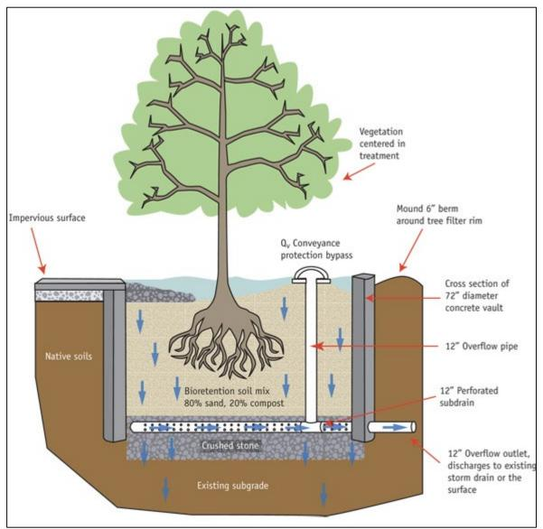
exiting the tree filter, either through an underdrain connected to the storm or combined sewer system or directly into underlying soils. The filter media removes a portion of pollutants carried by the runoff and stores moisture for use by the tree.
