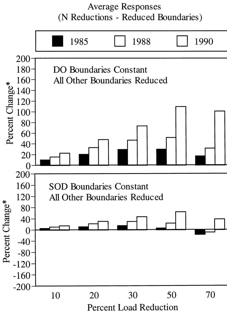
**FIGURE 3.37.** Predicted responses of average dissolved oxygen concentrations to nitrogen-loading reductions for different assumptions on seaward and bottom boundaries for 1985, 1988, and 1990 conditions.
