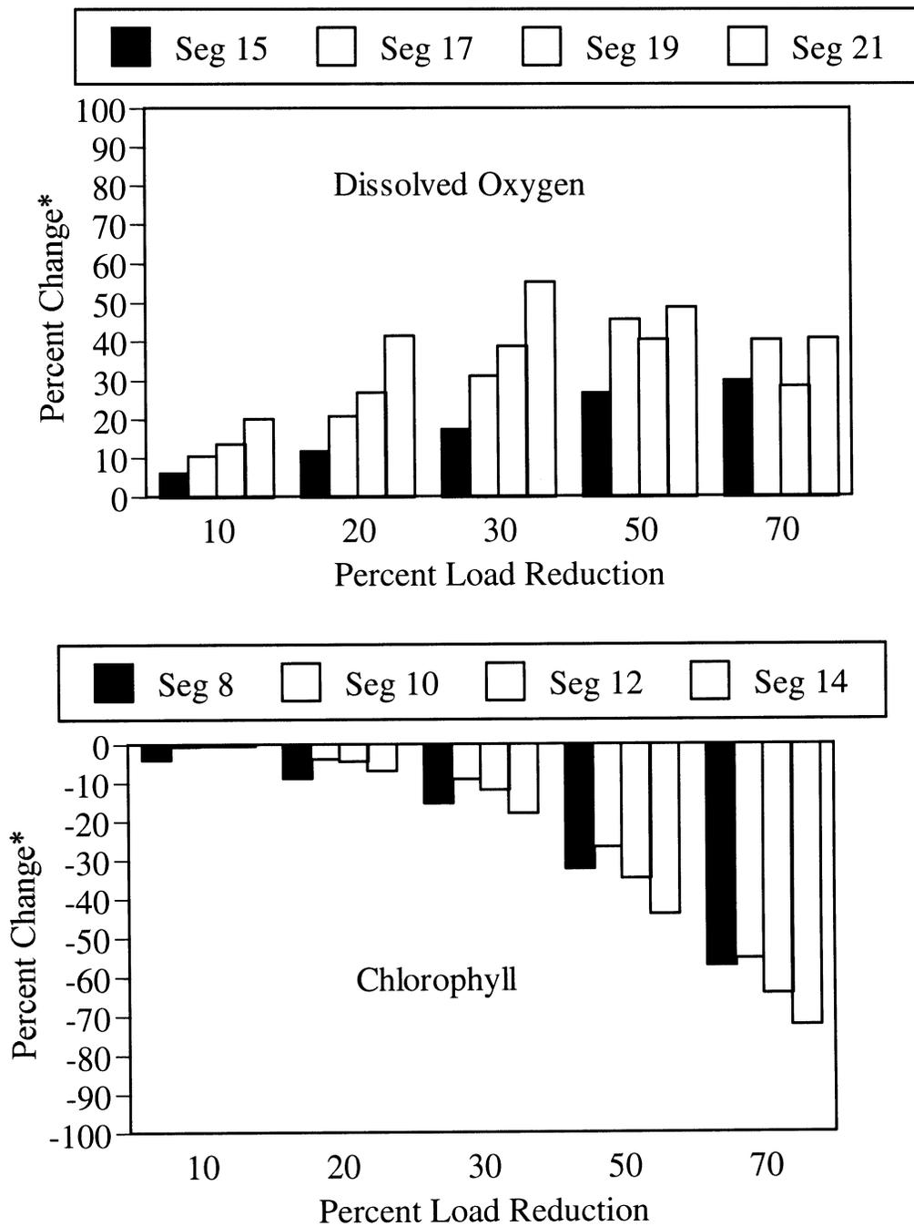
**FIGURE 3.40.** Predicted responses of average dissolved oxygen and chlorophyll concentrations for different spatial segments of nitrogen-loading reductions for 1985 conditions under reduced boundary conditions.
