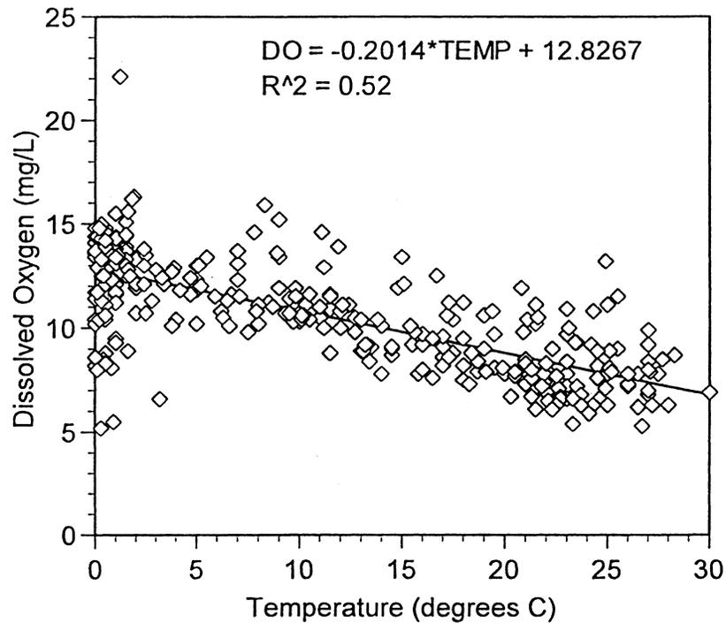
**FIGURE 3.20. Dissolved oxygen concentrations versus water temperature in the Minnesota River at Jordan for 1980–92.** NOTE: The dissolved oxygen saturation line is approximately equal to the shown regression line (DO saturation = 14.6 mg/L at 0°C, = 7.6 mg/L at 30°C). (Data from Metropolitan Council Environmental Services, St. Paul, MN.)
