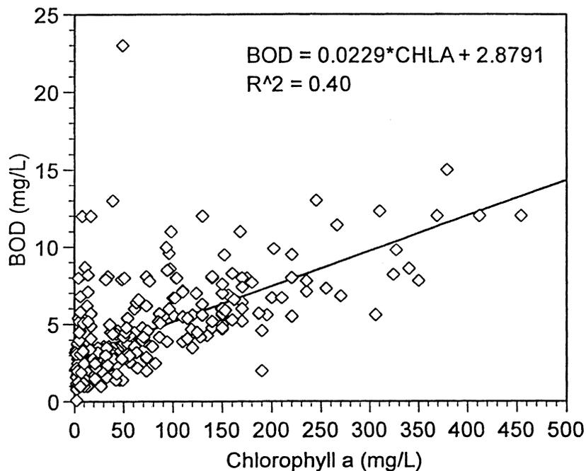
**FIGURE 3.21. Five-day biochemical oxygen demand (BOD<sub>5</sub>) versus chlorophyll a concentrations in the Minnesota River at Jordan for 1980–92.** NOTE: The highest measured BOD (23 mg/L) is from October 1989, during a drought with one of the lowest recorded discharge values (230 cfs). (Data from Metropolitan Council Environmental Services, St. Paul, MN.)
