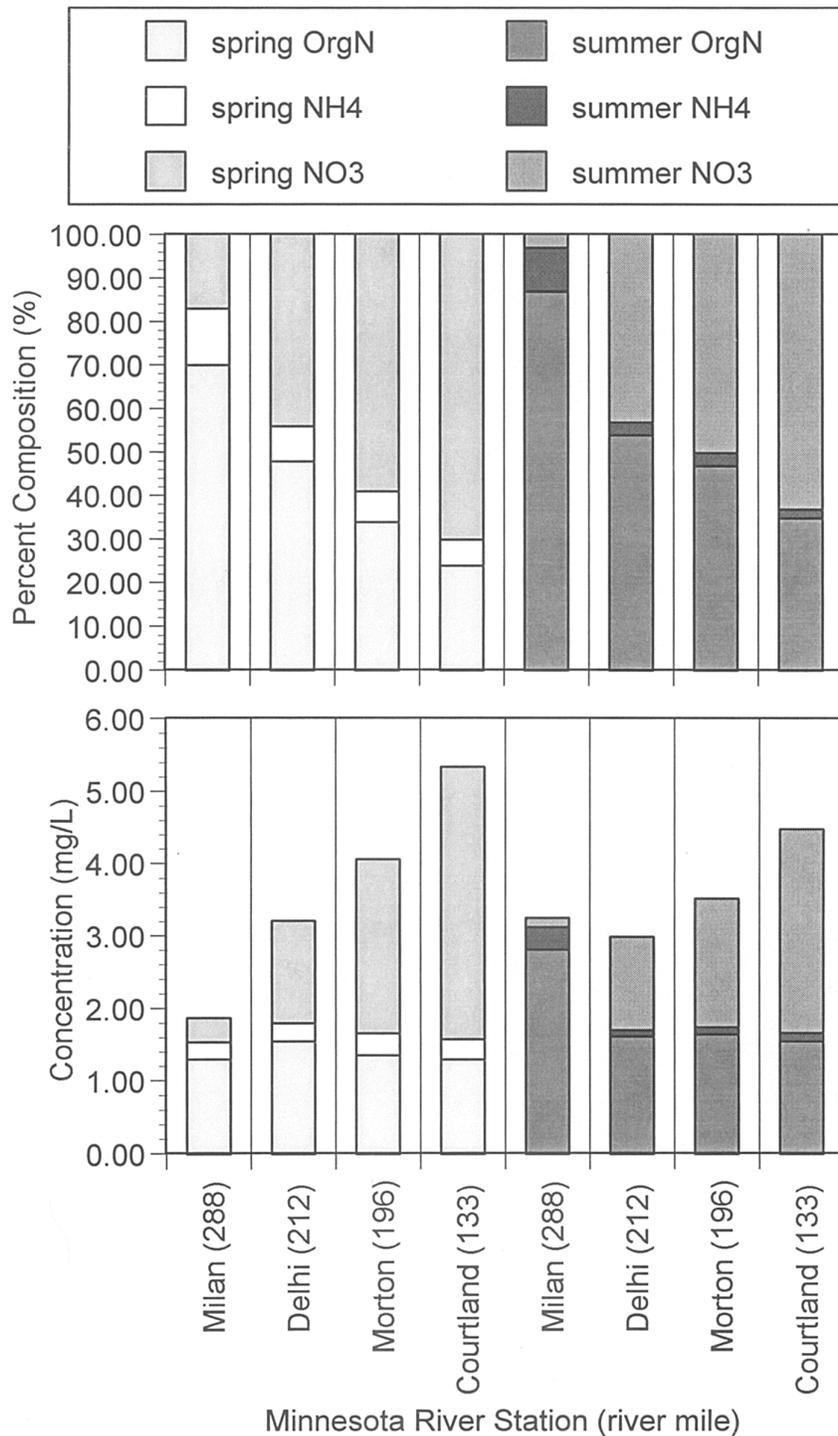
**FIGURE 3.19.** Percent composition (upper panel) and concentrations (lower panel) of nitrogen forms in spring (four bars to the left) and summer (four bars to the right) for four stations in the Minnesota River. NOTE: Stations are plotted left to right in order of downstream direction. (Data from various agencies and assembled by D. Mulla, University of Minnesota, St. Paul, MN.)
