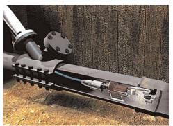
CISBOT Enters the Gas Main Via Its Launch Tube Attached to the Bidirection Fitting. Photo Courtesy of ULC Robotics.
