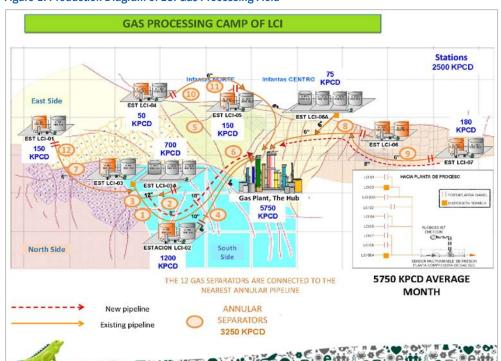
Figure 1. Production Diagram of LCI Gas Processing Field
