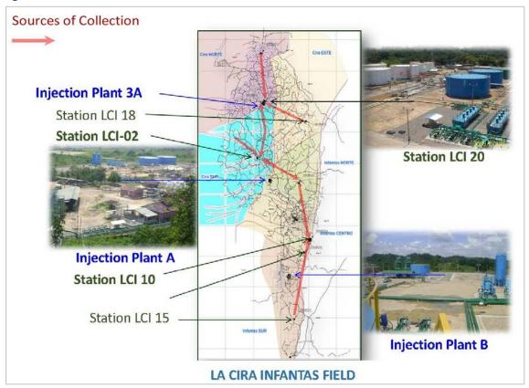
Figure 2 above shows the sources of gas collection at the LCI field. The scope of the project initially encompassed reducing casinghead gas emissions from 900 wells by 2013, and has since increased to a projected 1,000 wells by the end of 2015. The characteristics of vented natural gas directly correspond to gas chromatography samples entering the LCI processing plant.
