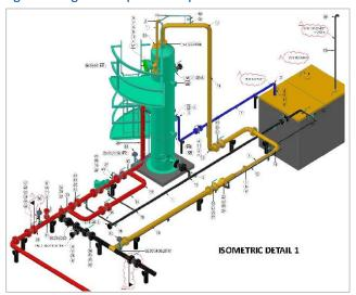
Image of a liquid gas separator
