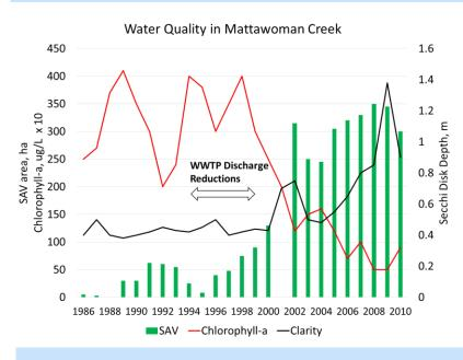
Phosphorus loads decreased significantly in the Bay watershed following the early 1980s ban on phosphorusbased laundry detergents. Yet, water clarity improved, chlorophyll levels dropped, and Bay grasses really began to rebound after wastewater treatment plant effluent was reduced as shown by the case Mattawoman Creek, above. Note: SAV data not available for 1988 and 2001. (bit.ly/ChesBayInsights)
