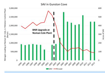
Wastewater treatment plant upgrades to BNR in the metropolitan Washington, D.C. area resulted in reductions in phosphorus and nitrogen concentrations. These nutrient reductions led to decreases in toxic cyanobacteria and helped submerged aquatic vegetation recover in the tidal Potomac River, such as those shown at Gunston Cove in Fairfax, Virginia. Note: 2001 and 2011 data not available. (bit.ly/ChesBayInsights)
