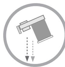
remove filter unit, turn up-side-down and gently tap out any debris after use
