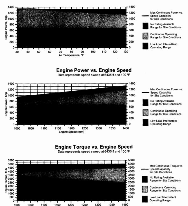
Note: At site conditions of 6435 ft and 100°F inlet air temp., constant torque can be maintained down to 1400 rpm. The minimum speed for loading at these conditions is 1000 rpm.
