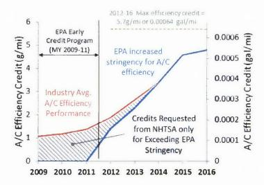
The blue line represents the amount of air-conditioner efficiency credits EPA projected for the fleet, including the stringency beyond the CAFE standards. The red line shows how the industry performed on average. The shaded area between the two shows the credits disregarded in the CAFE program, already accounting for the difference in the stringency of the standards.
