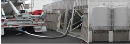
Weather permitting, raw material is delivered in a closed container and blown into Silo's via 4" diameter flexible metal pipe. All transfer operations are monitored visually by CPI Staff and all extraneous fugitive nurdles recovered (vacuumed) immediately.
