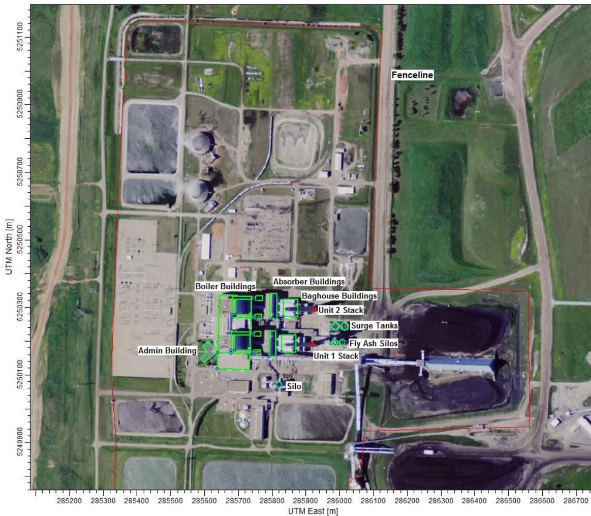
Figure 3-2: Stacks and Buildings Used in the GEP Analysis for Great Plains Synfuels Plant
