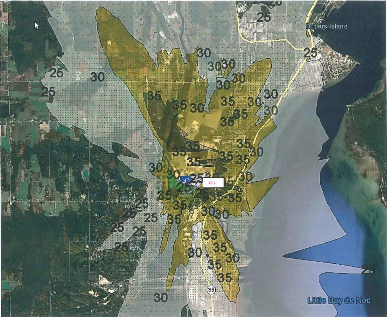
Figure 2. Isopleth and Maximum Impact (ppb) for Lafarge Cement (including background)
