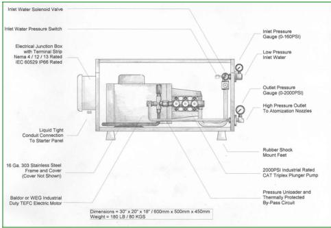
Belt Drive Pump Modules Above 5 GPM
