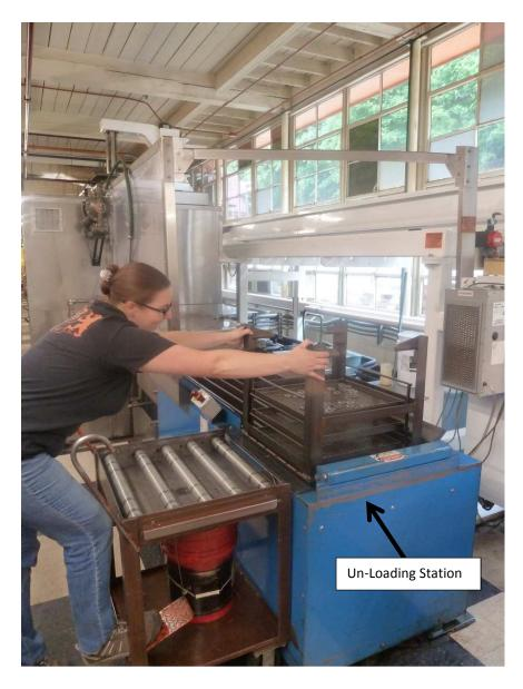
Greco Robot Actuated Degreasing System - Rear
