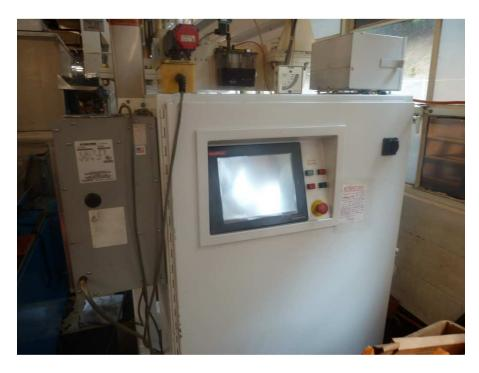
Greco Robot Actuated Degreasing System – Programmable Logic Control (PLC)
