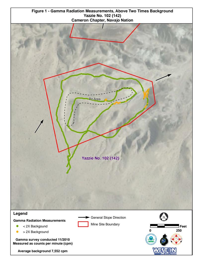
Figure 2 - Gamma Radiation Measurements Yazzie No. 102 (142) Cameron Chapter, Navajo Nation
