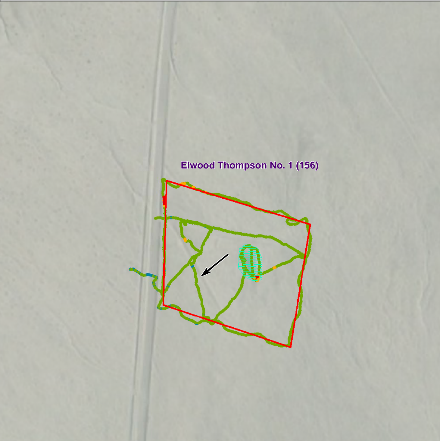
Figure 2 - Gamma Radiation Measurements Elwood Thompson No. 1 (156) Coalmine Mesa Chapter, Navajo Nation
