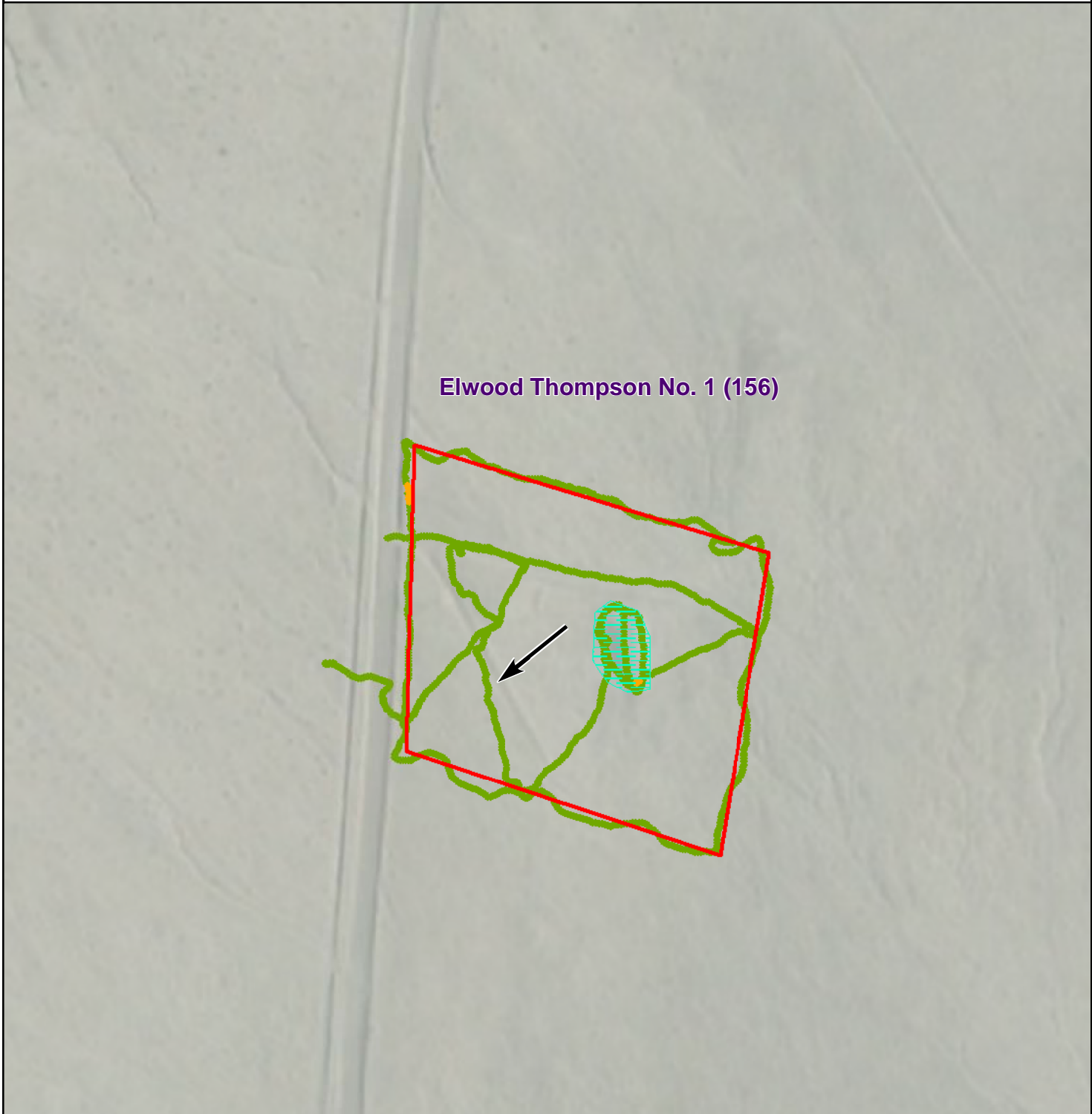
Figure 1 - Gamma Radiation Measurements, Above Two Times Background Elwood Thompson No. 1 (156) Coalmine Mesa Chapter, Navajo Nation
