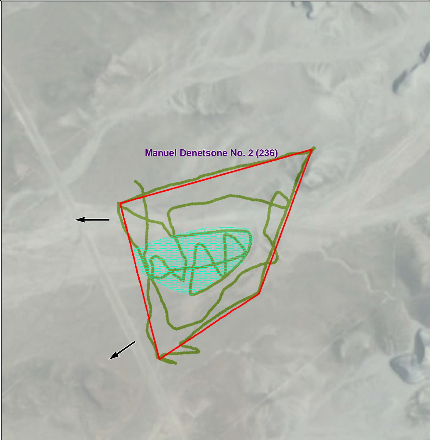
Figure 1 - Gamma Radiation Measurements, Above Two Times Manuel Denetsone No. 2 (236) Coalmine Mesa Chapter, Navajo Nation
