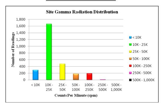
**Highest gamma radiation measurement:** 148,871 counts per minute (cpm)
