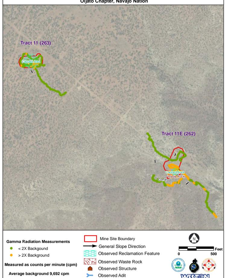
Figure 2 - Gamma Radiation Measurements Tract 11 and Tract 11E (262, 263) Oljato Chapter, Navajo Nation
