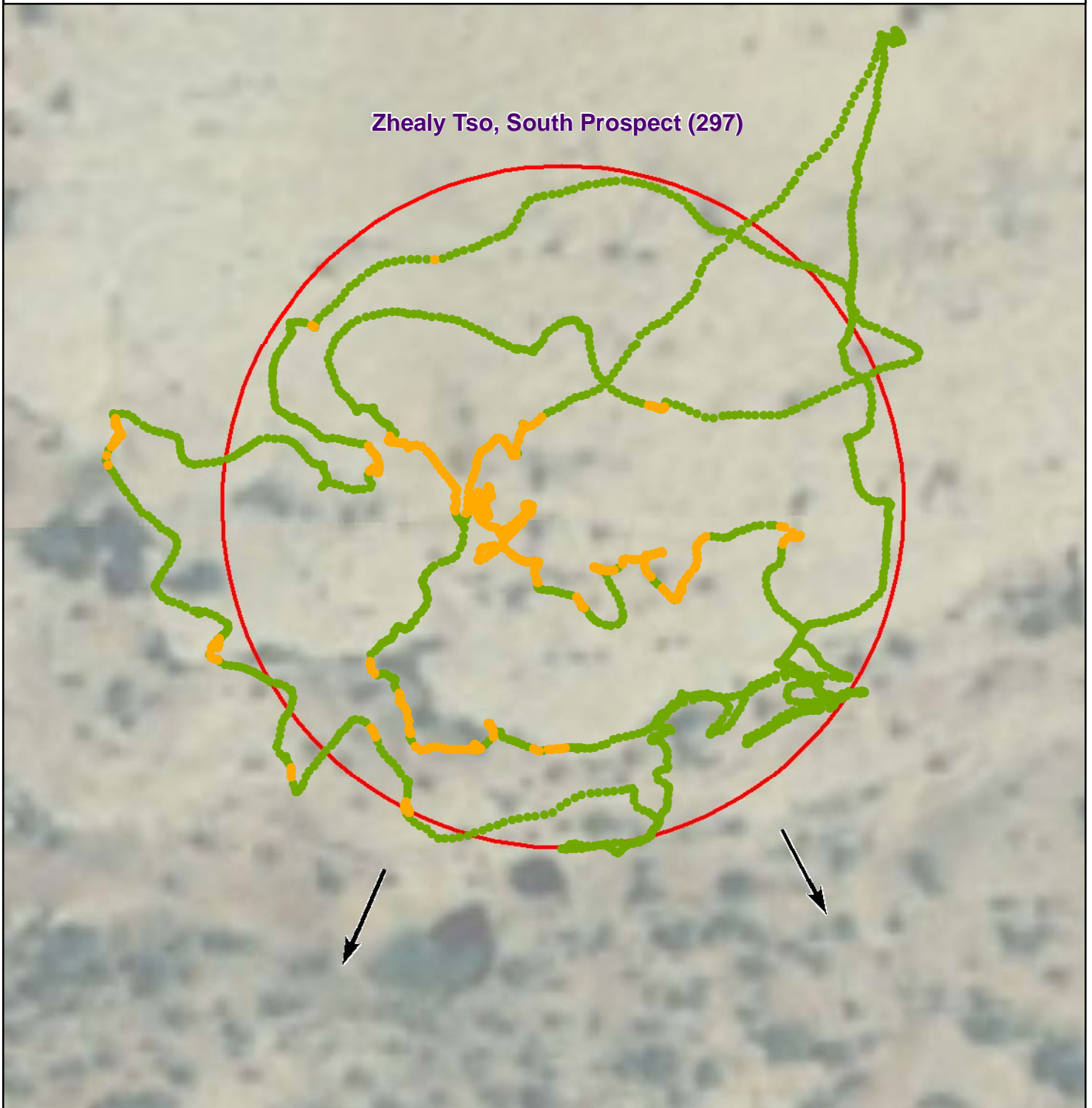
Figure 1 - Gamma Radiation Measurements, Above Two Times Background Zhealy Tso, South Prospect (297) Chinle Chapter, Navajo Nation
