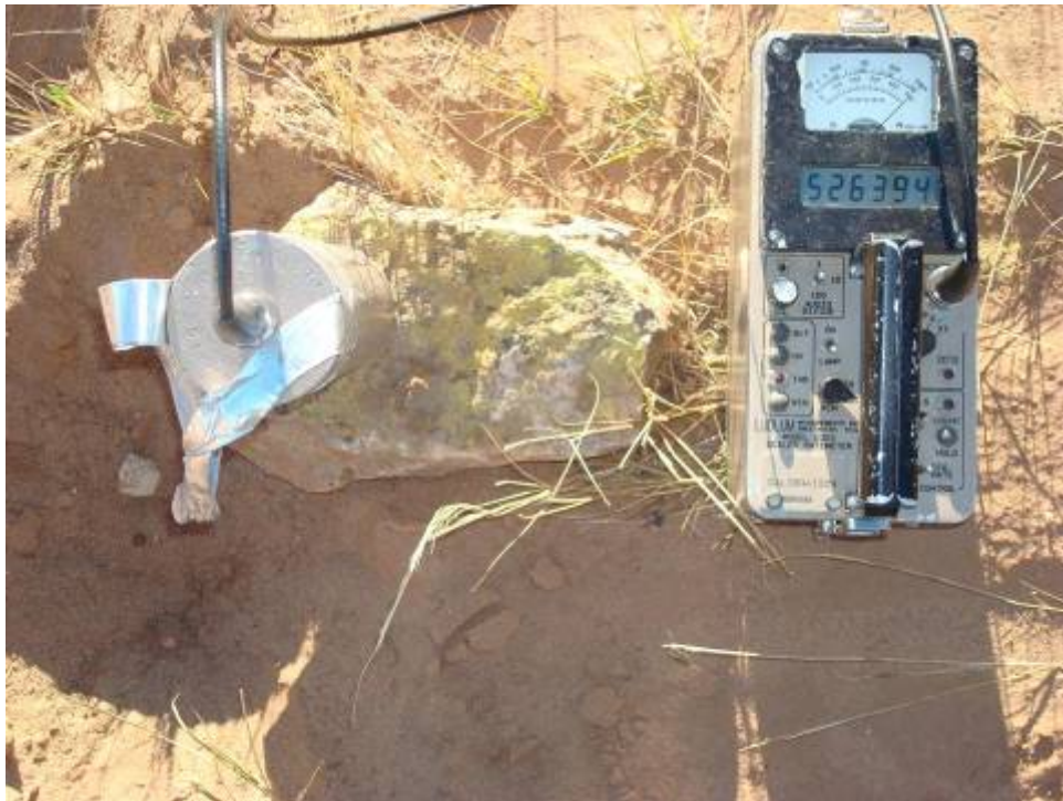
Photo 6. Haystack No 1 Mine site, gamma radiation emitting 500,000 cpm from waste rock located near residence
