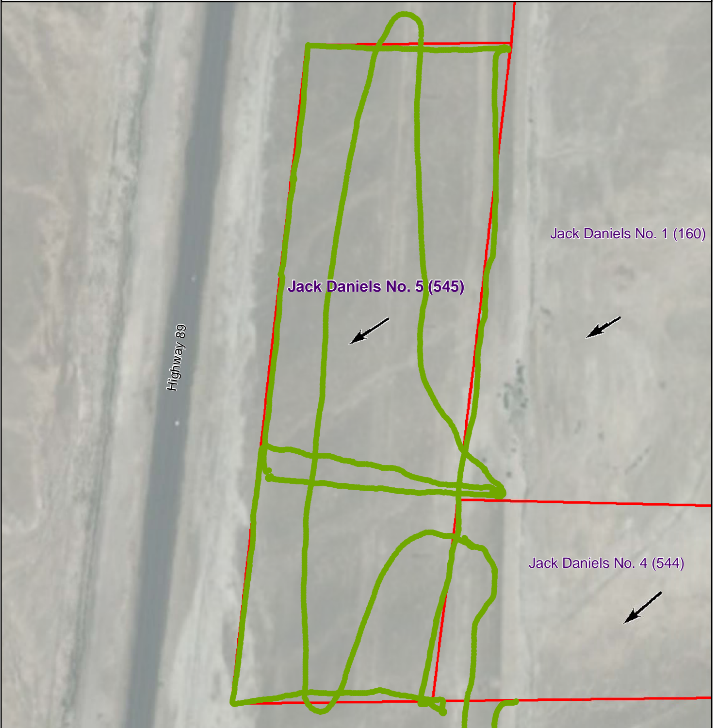
Figure 1 - Gamma Radiation Measurements, Above Two Times Background Jack Daniels No. 5 (545) Coalmine Mesa Chapter, Navajo Nation
