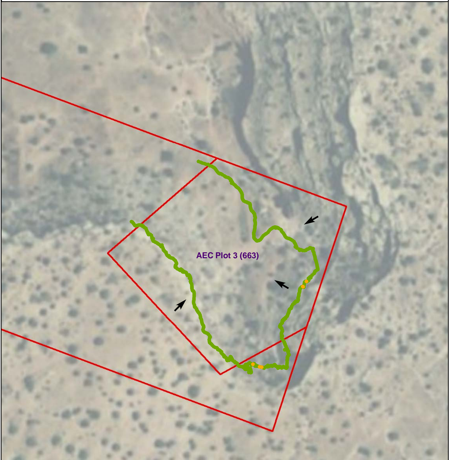
Figure 1 - Gamma Radiation Measurements, Above Two Times Background AEC Plot 3 (663) Sweetwater Chapter, Navajo Nation
