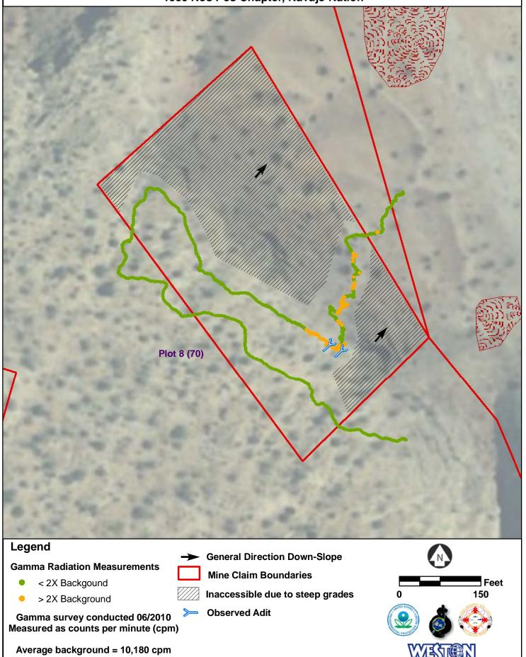
Figure 2 - Gamma Radiation Measurements Plot 8 (70) Teec Nos Pos Chapter, Navajo Nation
