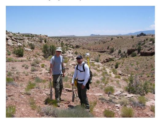
Photo 4: WESTON used a combination sodium-iodide scintillation detector and a GPS unit (right). A stand-alone scintillation detector also was used (left).
