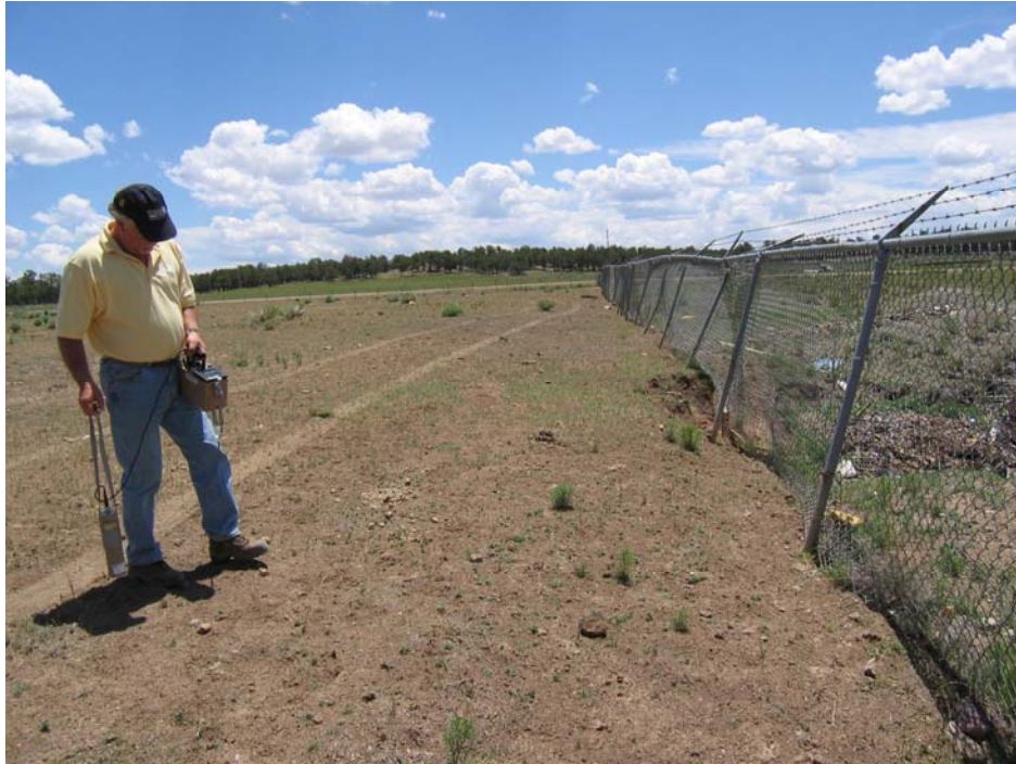
Photo 3: WESTON collecting gamma radiation readings with a sodium-iodide scintillation detector.
