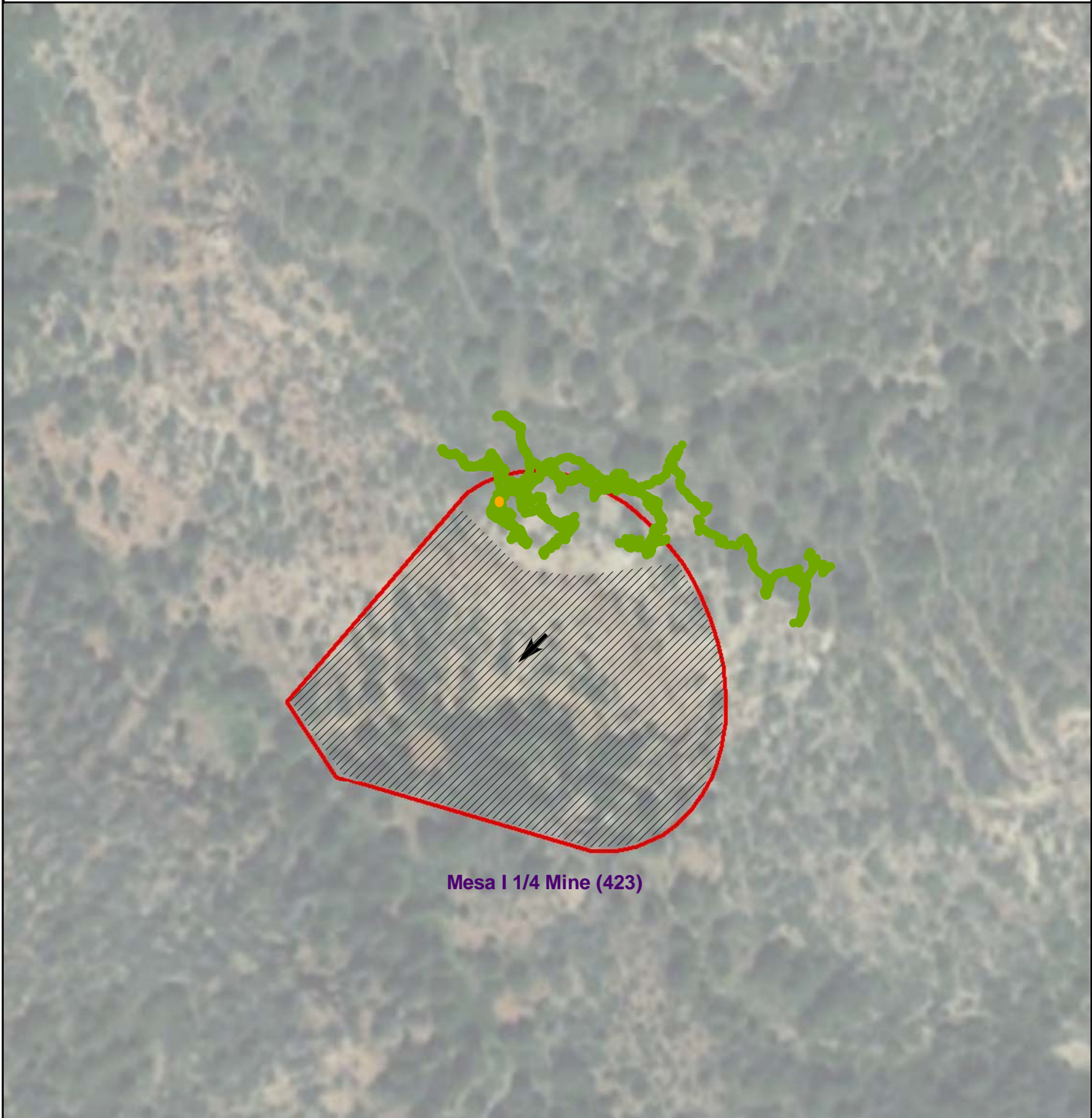
Figure A-6 - Gamma Radiation Measurements, Above Two Times Background Mesa I 1/4 Mine (423) Cove Chapter, Navajo Nation
