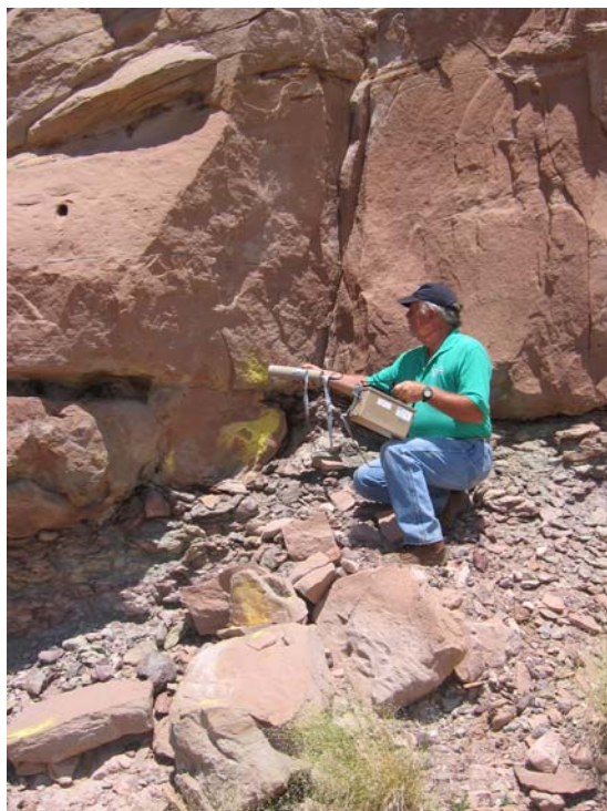
Photo 2: WESTON employee holds sodium-iodide scintillation detector to exposed uranium ore at Mine 12.
