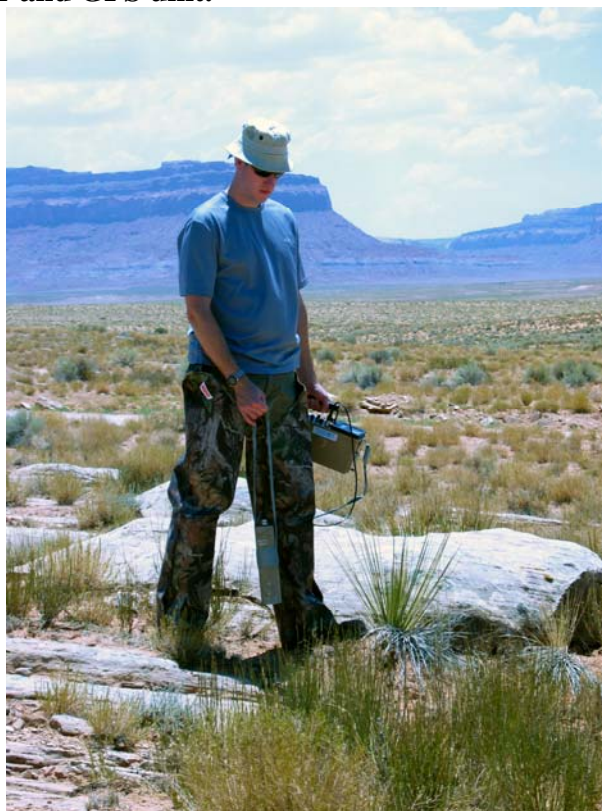
Photo 3: WESTON collecting gamma radiation readings using a combination scintillation detector and GPS unit.
