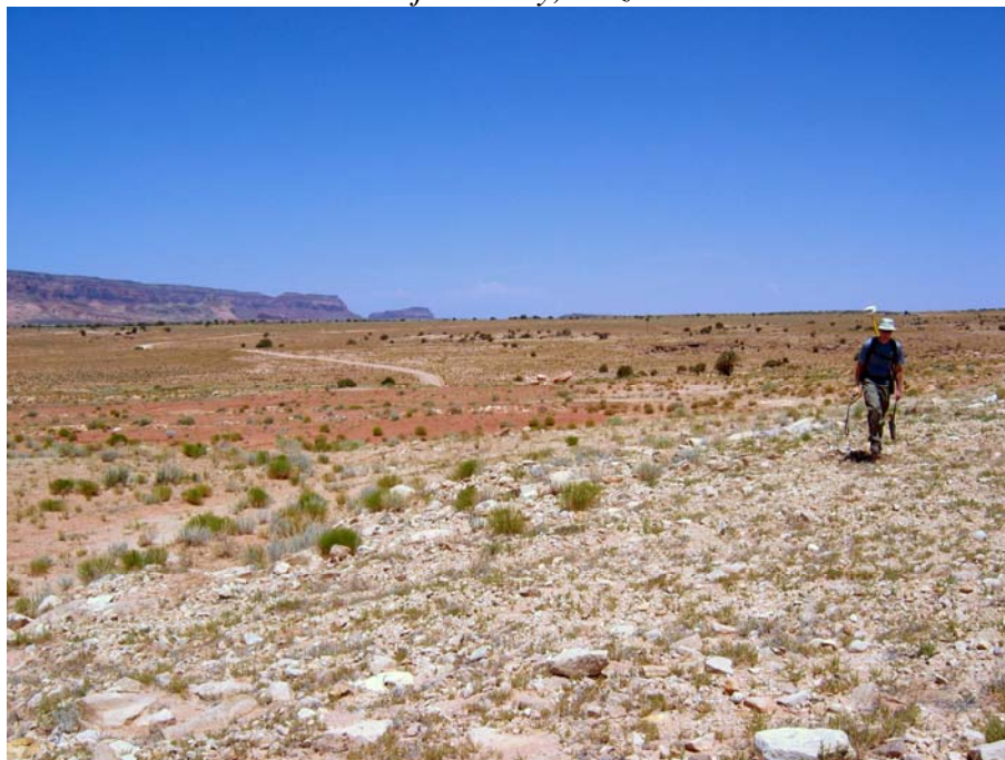
Photo 3: WESTON collecting gamma radiation readings using a combination scintillation detector and GPS unit.
