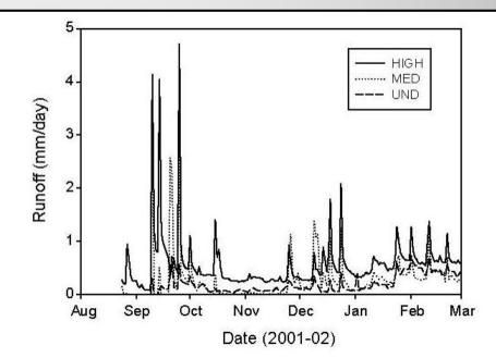
Figure 33. Stream runoff during a dry period (Aug 2001-Feb 2002) at three study catchments: UND = undeveloped, MED = medium density residential (1.6 houses ha<sup>-1</sup>, 6% impervious), HIGH = high density residential (2.8 houses ha<sup>-1</sup>, 11% impervious).
