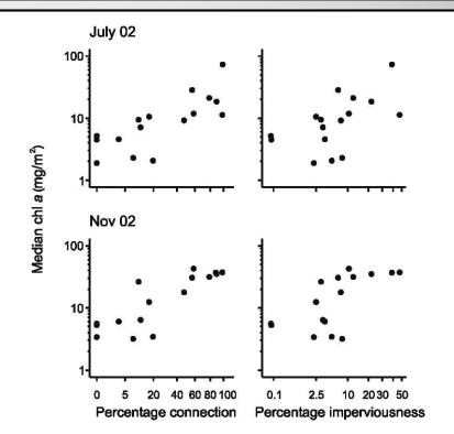
Figure 44. Median chlorophyll *a* at 16 Australian streams on 2 sampling dates, vs. % drainage connection and % imperviousness; % connection (but not % imperviousness) explained a significant amount of variation in chlorophyll *a* in both sampling periods.
