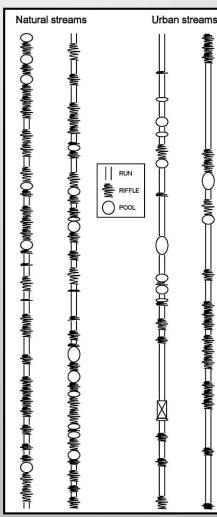
Figure 38. Schematic representation of the run, riffle and pool structure in two natural & two urban streams in southern California (the rectangle with an X in one of the urban streams represents a culvert). Urban streams had longer habitat segments, higher percentages of runs, & reduced habitat complexity.
