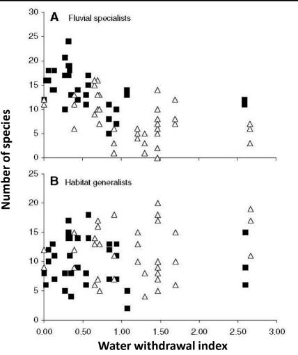
Figure 36. Richness estimates for (A) fluvial specialist and (B) habitat generalist fishes vs. water withdrawal index values [In(permitted monthly average withdrawal / 7Q10)]. Squares indicate sites where water intake was directly from channel; triangles indicate sites directly downstream from water supply reservoirs. Data were collected in 28 Georgia streams used for municipal water supplies, 2001-2003.
