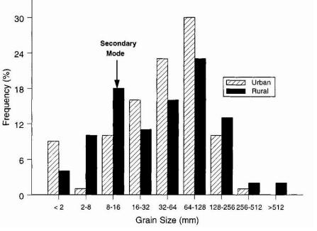
Figure 39. Typical grain-size histograms from urban and rural catchments. The frequency of < 2 mm particles more than doubled in urban streams. Rural streams had a secondary sediment size mode at 8-16 mm; this secondary mode was absent in urban channels, suggesting that these substrate sizes were selectively removed from urban streams.
