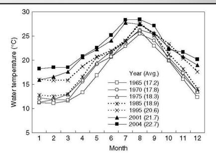
Figure 26. Monthly mean (plot) and yearly mean (legend) temperatures of wastewater effluents from all treatment plants located in the central Tokyo area, 1965-2004. Increases in effluent temperatures stem largely from increased residential use of heated water.
