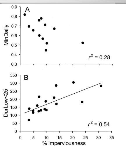
Figure 35. Linear regression models for baseflow variables showing highest correlations with subcatchment imperviousness: (A) minimum daily stage/mean daily stage during late spring; (B) maximum duration of low stage <25<sup>th</sup> percentile during autumn. Of the nine baseflow variables tested across five seasons, only these two variables showed relationships with r<sup>2</sup> > 0.25, and only in (B) was this relationship significant.
