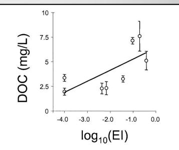
Figure 45. Relationship between catchment effective imperviousness (EI) and dissolved organic carbon (DOC) concentration in eight streams east of Melbourne, Australia ( $r^2 = 0.05$ , p = 0.051).
