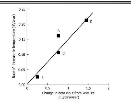
Figure 27. Change in wastewater heat effluent from wastewater treatment plants vs. the rate of temperature increase in four stream segments (B-E) in the Ara River system, central Tokyo. Kinouchi et al. (2007) contend that increased wastewater effluent temperatures contribute to the thermal degradation of effluent-receiving streams.
