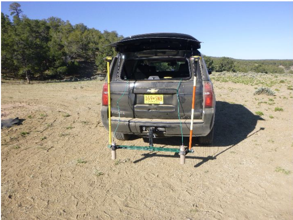
Photo 17: Radiological Survey using Vehicle Attachment
