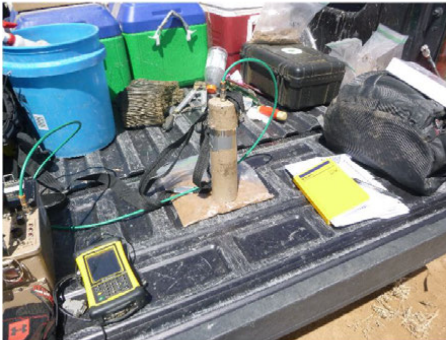
Photo 19: Background Soil Sampling - Performing Static Measurements for Soil Samples
