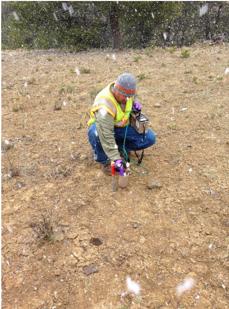
Photo 18: Correlation Soil Sampling - Static In-Situ Measurement
