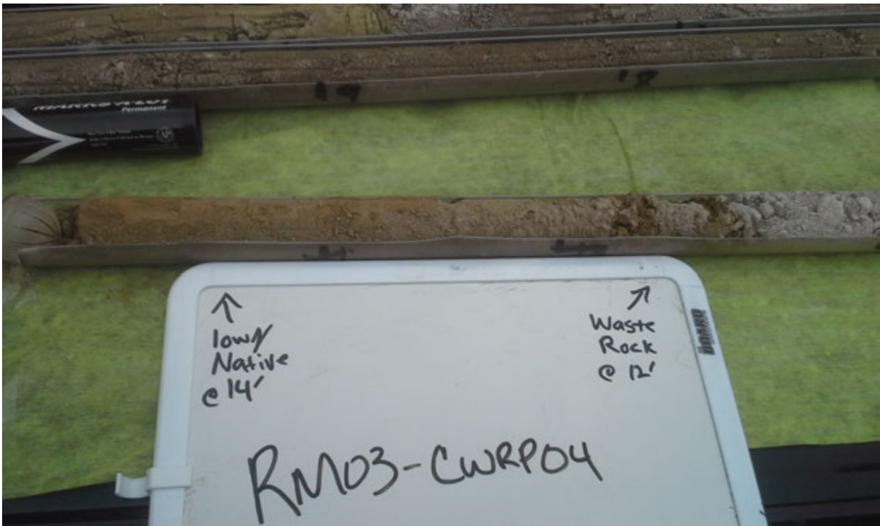
Photo 26: Soil Core Screening Indicating Transition from Waste Rock to Native Soil (Boring RM03-CWRP04 with Bottom at Left)
