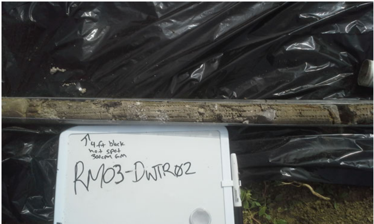
Photo 25: Soil Core Screening Indicating Subsurface Waste Rock (Boring RM03-DWTR02 Core)
