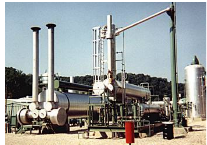
Glycol Dehydrator Unit Source: GasTech
