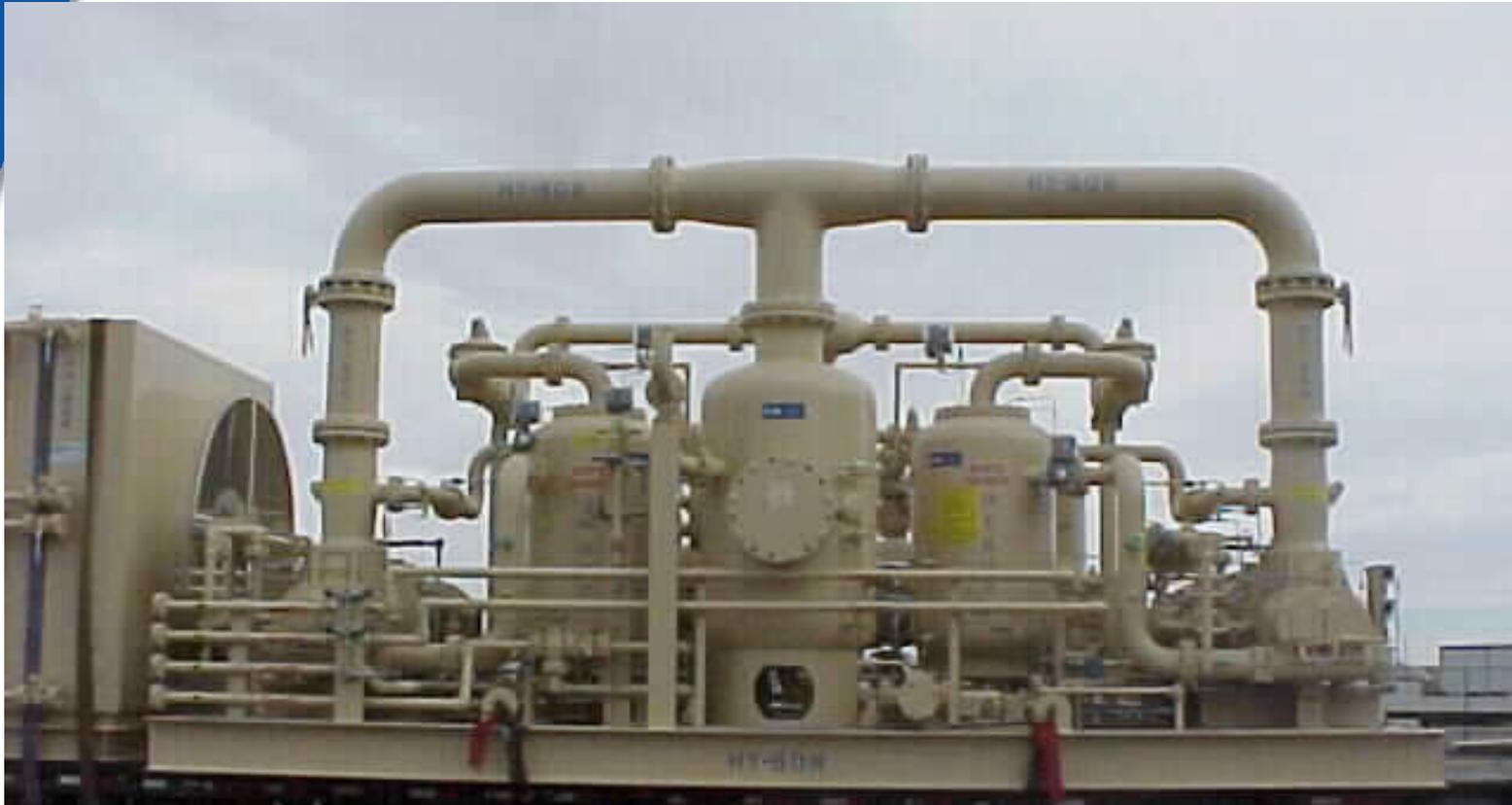
*This dual flooded screw package for PDVSA is designed for volumes to 0,14 MMm<sup>3</sup>D; moving tank vapors from 0 to 14 kg/cm<sup>2</sup> in Eastern Venezuela.*
