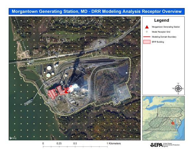
Figure 4. Fence Line Receptors for the Morgantown Generating Station
